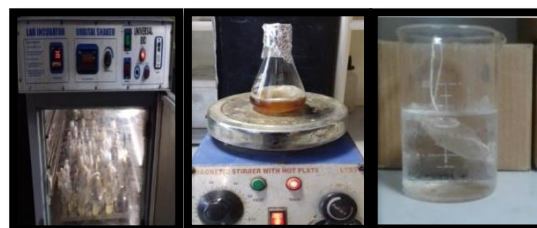
Figure 5: fermentation of nattoxinase and its purification by salt precipitation and dialysis.
